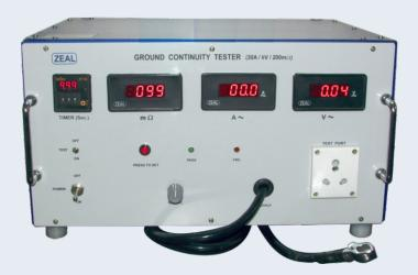
The Ground / Earth continuity tester works with the test current of the sinusoidal waveform. The typical test current severity is 30A. Meters indicate test current, the voltage drop across the ground path, and  $m\Omega$  resistance of the ground path. The main purpose of this test is to detect a totally open or loose ground connection.
