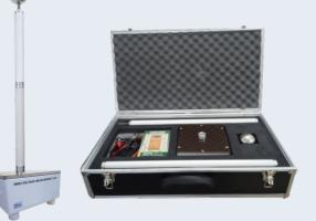
'Zeal' AC /DC High Voltage Measurement probe along with handheld Digital Multimeter is an essential combination to measure the output of High Voltage Transformers, High Voltage Testers, High Voltage Power Supplies, etc. The attenuation ratio is reasonably sufficient. The output accuracies for both DC & AC HV measurements are excellent.
