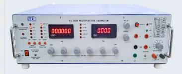
The Multi-Function Calibrator is useful for the calibration of Digital Multimeters, Clamp Meters, Digital Panel Meters, Analog Panel Meters, LCR Meters & Non-Contact Type Tachometers. It is a variable source with different ranges of DC Voltage, AC Voltage, DC Current, AC Current, Frequency, Resistance, Capacitance, Inductance & RPM (Non-Contact Type). It has been designed to calibrate the maximum ranges of a variety of models of multimeters available in the market.
